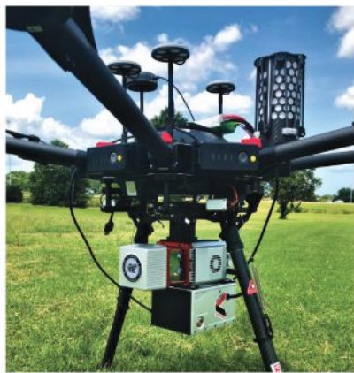
THE PARACHUTE rests in the cannister attachment on the UAV's upper right.
